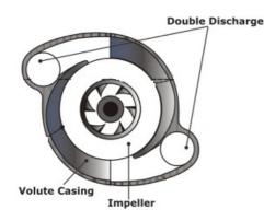
This figure show how the thrust is balanced by the Twin-Volute with 180 degrees opposite discharge outlets.
